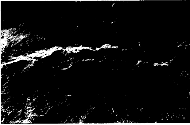
Fig. 12. Photomicrograph of a subsurface crack on fracture surface of a specimen after binder removal to 220°C at a heating rate of 10°C h -1 in oxygen.
